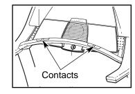
sensor, with your palms on the metal contacts. Avoid moving your hands. When your pulse is detected, two dashes (--) will appear in the Calories/Pulse display, and then your heart rate will be shown. For the most accurate heart rate reading, continue to hold the contacts for about 15 seconds.
